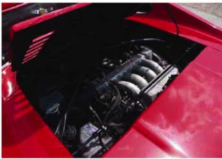
The 2-litre 16-valve, 35-0C engine develops 158 bhp although later cars had more power (up to 172 bhp). The turbo models were not sold in Europe but there are plenty of grey imports around.
