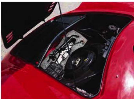
The front compartment is all business with the spare wheel, tools, master-cylinders and electrics but there's still room for a few odds and ends.
