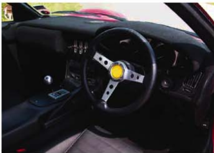
Replica heater slide controls and switches on centre dash are dummies. There's no Prancing Horse on the wheel boss or anywhere else as the car never carried them. It was marketed as a Dino.
